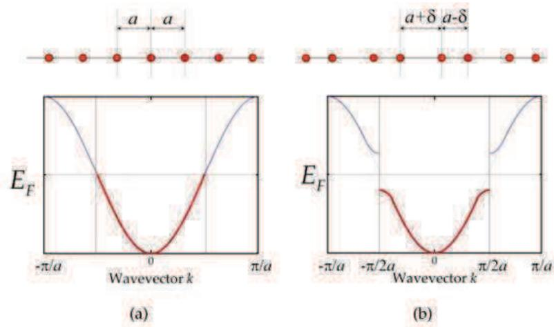
Peierls distortion ([https://www.utwente.nl/tmw/pin/onderzoek/physical\\_properties\\_of\\_low-dimensional\\_systems/physical\\_properties\\_of\\_low-dimensional\\_systems-8.png](https://www.utwente.nl/tmw/pin/onderzoek/physical_properties_of_low-dimensional_systems/physical_properties_of_low-dimensional_systems-8.png))
